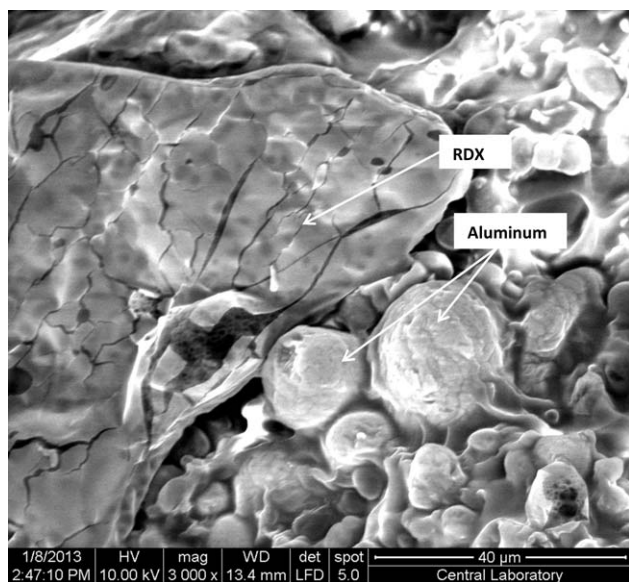
Figure 5. SEM image of explosive containing DOA as a plasticizer.
